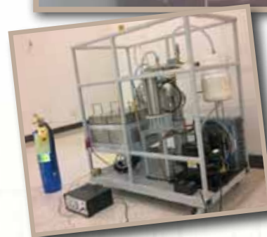
The prototype of 1 kW-hydrogen generator developed in the laboratory
